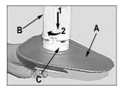
Reassemble the filter parts (as shown in the figure) and reinsert the whole assembly into the dishwasher. Position it into its housing and press downwards. The dishwasher is not to be used without filters. Improper replacement of the filters may reduce the efficiency of the wash and even damage your dishwasher.
